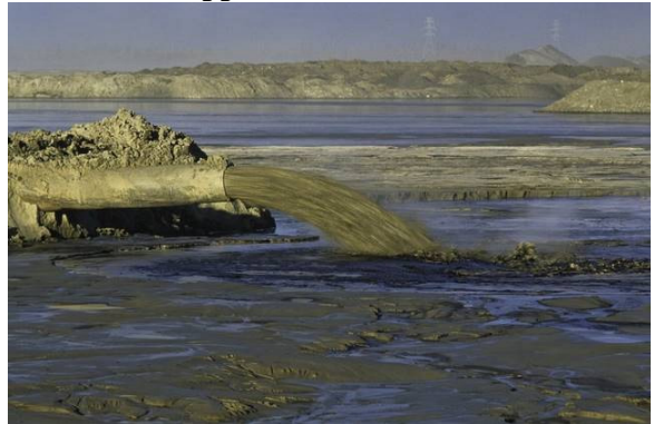
AN EFFLUENT PUMP DUMPS MINE TAILINGS AT ONE OF SYNCRUDE’S TAILINGS POND SITES
